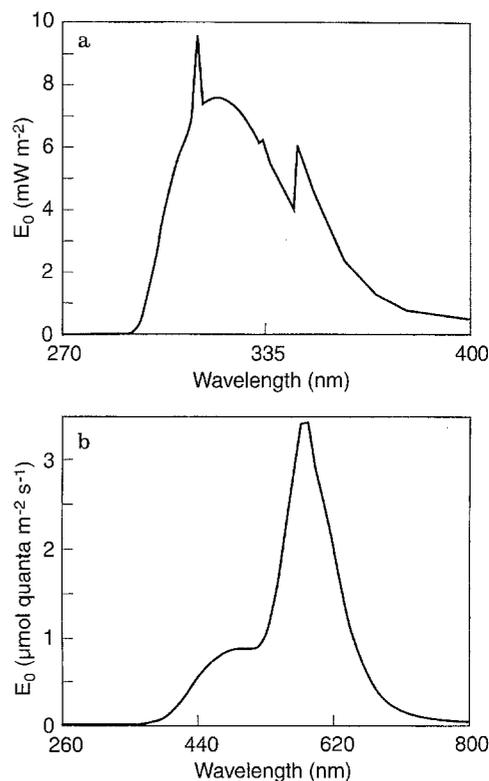
**Fig. 1** Spectral irradiance ( $E_0$ ) of lamps used in all experiments. **a** Westinghouse FS-40 Sunlamp with maximum emission at 313; **b** GE cool-white PAR lamp with emission peak at 580 nm
