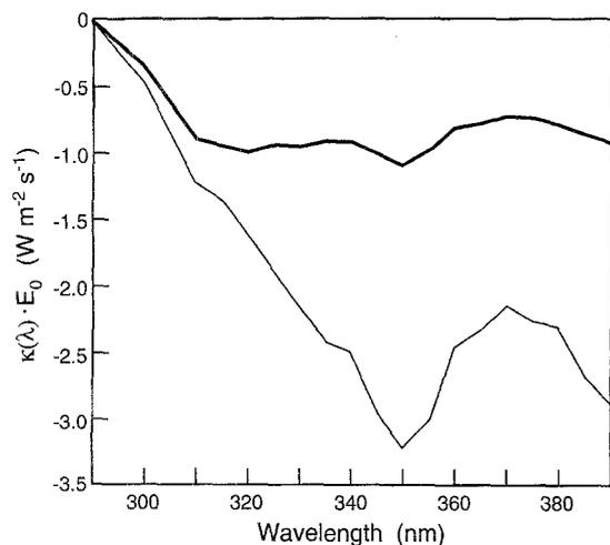
**Fig. 7** Photooxidation rate constants [ $\kappa(\lambda)$ ,  $\text{s}^{-1}$ ] over 48 h of experiment, as estimated by Kouassi and Zika (1992) as a function of wavelength for Experiments 2 (thick line) and 3 (thin line)
